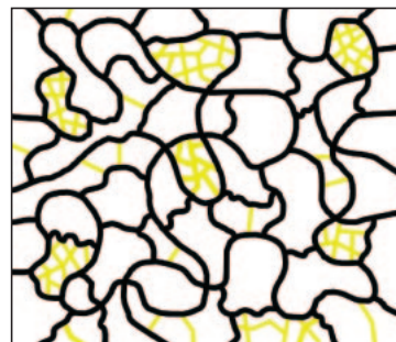
Fig. 4. Schematic illustration of the interpenetrated network of organic (in black) and inorganic (in yellow) components.
